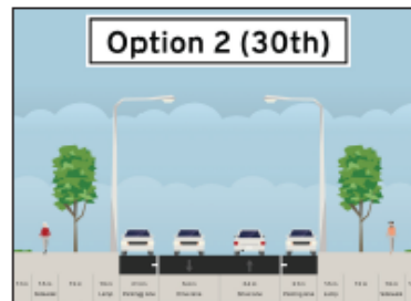
30th Street shown as a "minor collector" as per City of Lethbridge specifications, with separated sidewalks and boulevards on each side.
